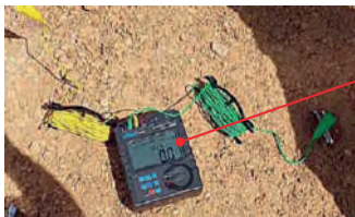
2 Wires earth voltage test: result: 0 Volt
