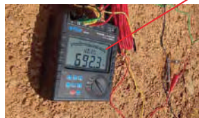
2 Wires resistance test: result: 9,54 \Omega
