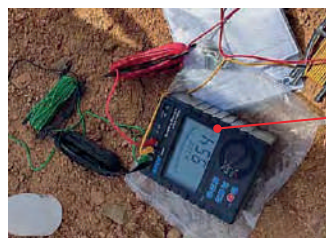
2 Wires resistance test: result: 9,54 \Omega
