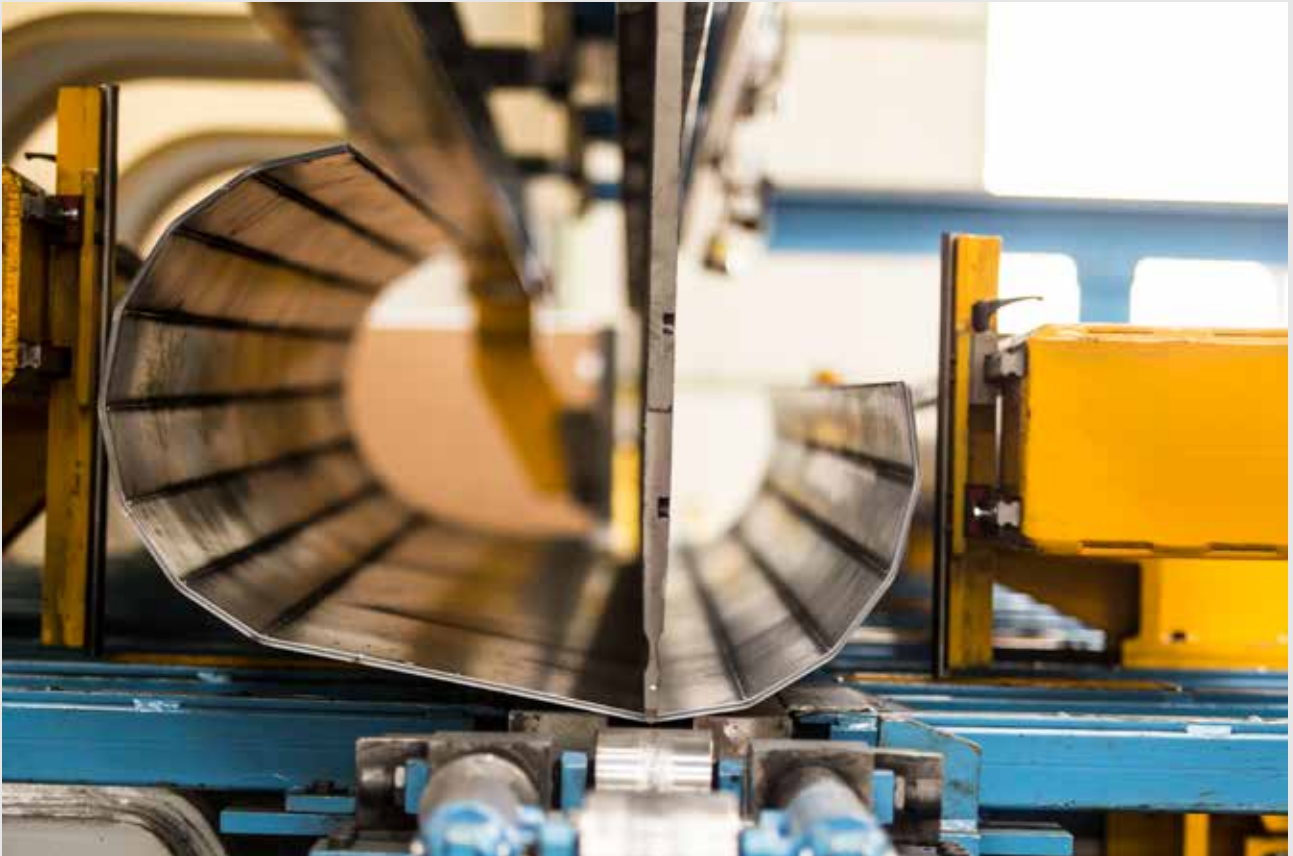
Steel sheet stamping process in a 14 mt automatic bending machine
