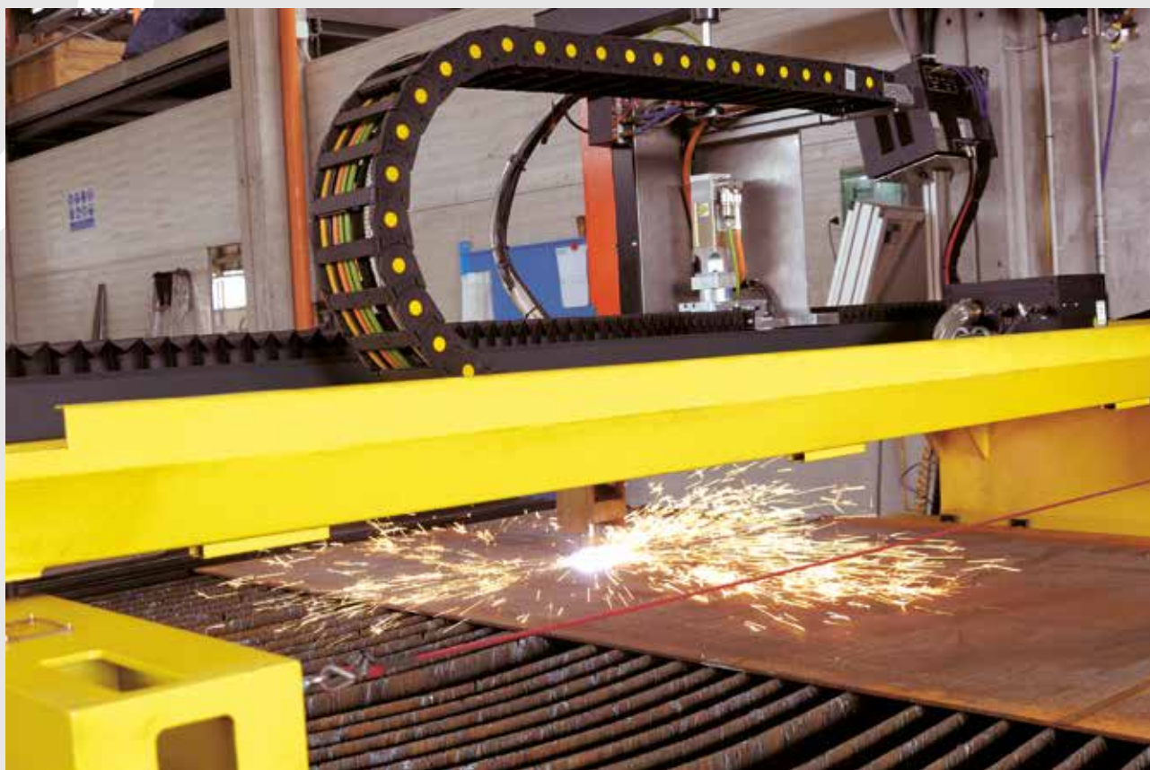
Steel sheet cutting with high definition plasma machine
