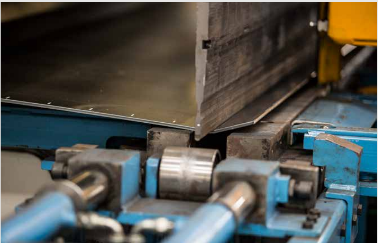
Steel sheet stamping process in a 14 mt automatic bending machine
