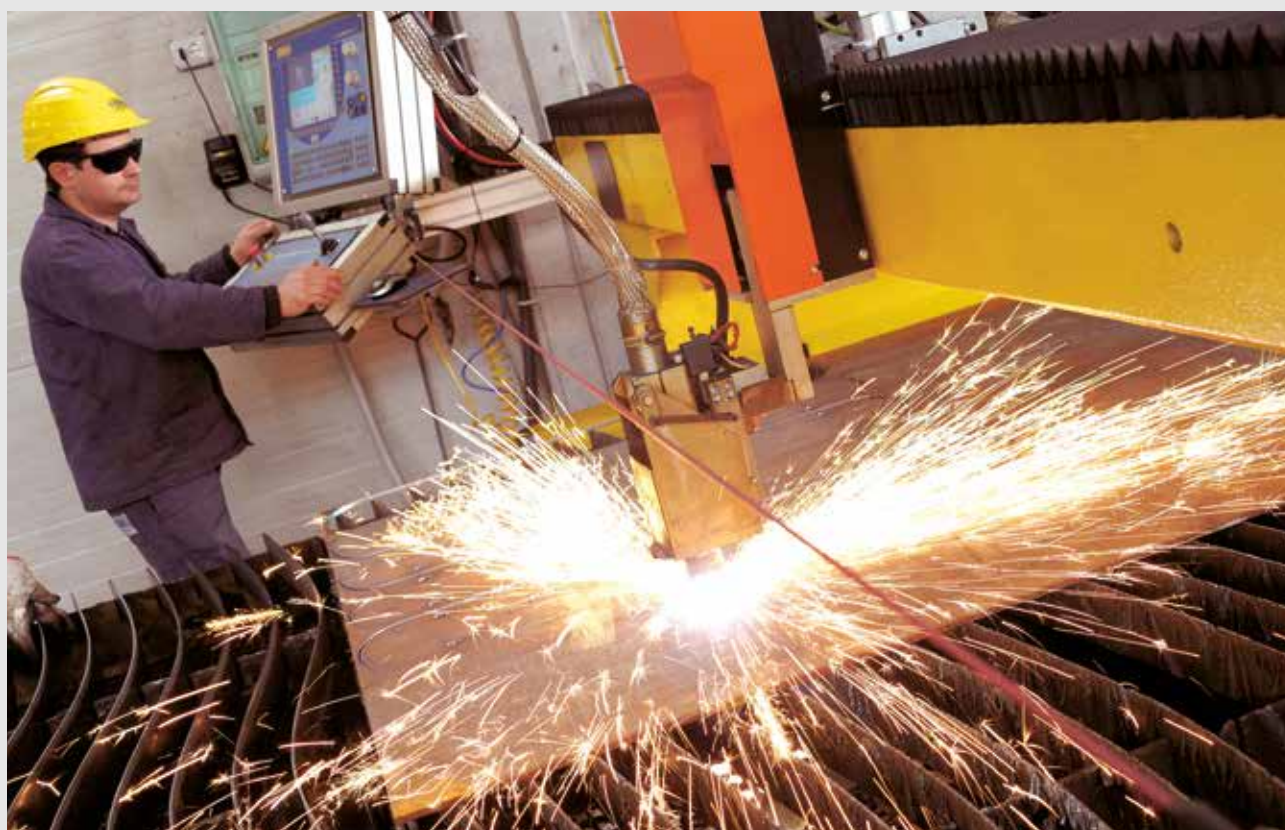
Steel sheet cutting with high definition plasma machine
